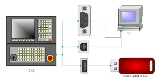
CNC can transfer data betweenPC and CNC via serial port (RS232C) or by USB (in CNC20 there Is embedded converter USB-RS232). Driver for windows is included in CD:
